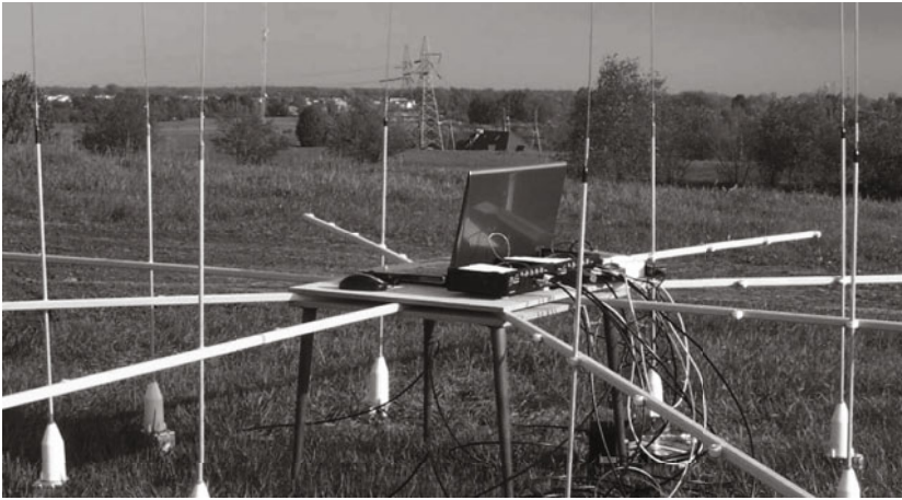
Fig. 7. Multichannel signal receiving and processing SDR-based platform
