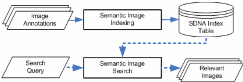
Fig. 2. Conceptual diagram showing the process flow of Semantic Image Indexing and Semantic Image Search
