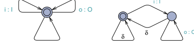
Fig. 5. A trivial learning purpose (left) and a learning purpose with a nontrivial \delta transition (right)
