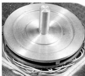
Fig. 10.28 Mode rotary type step USM using 5-phase driver
