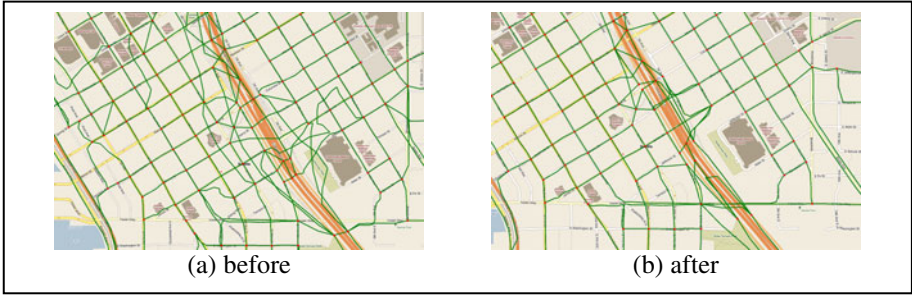
Fig. 7. After connecting the intersections using the road filling algorithm, there are some mistaken connections. In (a) we have shown the road network before pruning incorrect connections. In (b) the road network is depicted after removing incorrect connections.
