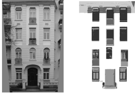
Fig. 6. left (Exp. 1): Classification rate obtained by 10-fold cross-validation. "BCH" shows the probabilistic context based on the position alone, "DT" the class probability based on appearance features estimated by the decision tree, the last column shows the combined result. Fig. 6 middle and right (Exp. 2): Facade image (middle) and result of context-based segmentation (right). The BCH used six structural models, out of which the most fitting one was automatically selected and used to interpret the polygons provided by the low level.
