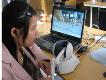
Fig. 3. User interacting with the haptic virtual environment using a PHANTOM Omni force feedback device (source: SensAble Technologies Inc)
