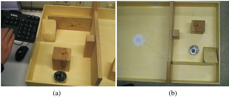
Fig. 3. Implementation. (a) demonstration made on the robot learner. (b) after training, the ESN controls the robot.
