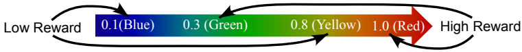
Fig. 4. Nonlinear Reward Color Encoding. The agent receives a high reward for green or red and a low reward for blue or yellow. The ANN color encoding together with the given ANN topology requires the agent to include a nonlinear learning rule.
