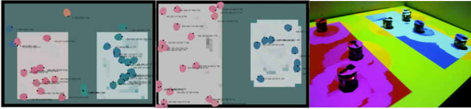
Fig. 4. Final multirobot system obtained for two different cases. The left image corresponds to the result obtained when the areas have the same size and the central one when the size of the area to be mowed is increased. The colors of the robots on the computer view represent genotype and the color intensity in each area the level of grass/leaves. The right figure shows a view of the experimental setup with 8 e-puck robots.
