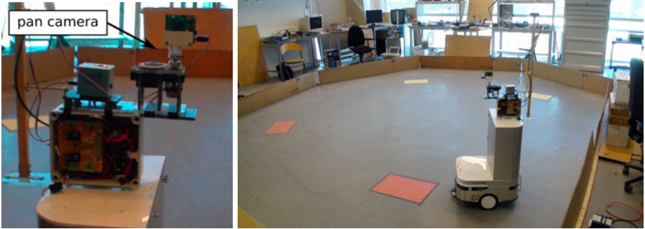
Fig. 1. The robot in its environment (equipped with a color detector placed under it). Colored squares on the ground are simulated resources.
