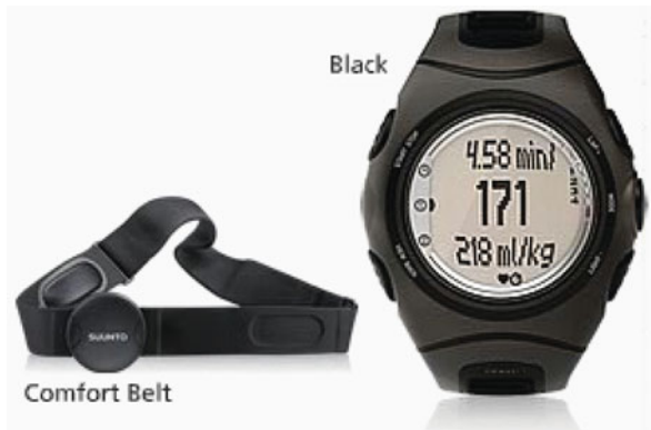
Fig. 6 Watch with wireless ECG-derived heart rate monitor ( www.suunto.com )
