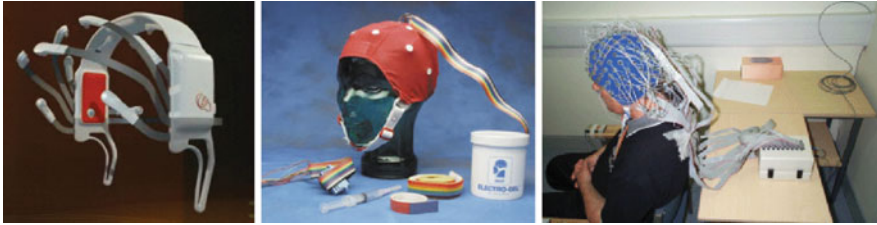
Fig. 13 Three examples of the range of electrode quantity found in EEG interfaces. From left to right : the emotivEpoc ( www.emotiv.com ), a standard 10–20 EEG array ( www.biopac.com ), and a 256 lead array ( www.biosemi.com )
