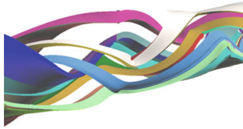
Fig. 8. Visualization of several stream volumes. A stretching, rotating and diverging motion between adjacent volumes can be observed.
