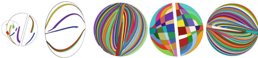
Fig. 10. Slicing planes through five (left) and all volumes of the data set (right) at positions t = 0.3, 0.6, 1.0, 0, 0.5, 1.0 . It is clearly visible, how neighboring volumes take different paths through the data set. Comparison between individual slices allows observation of stretching, rotational, and mixing behavior. The distribution of volume colors indicate a good mixing process.
