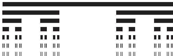
Fig. 8.1 Construction of the “middle-third-erasing” Cantor set: The replication rule is to eliminate the middle third of every bar in subsequent subdivisions. The total length converges to zero, while the fractal dimension is D = \log(2)/\log(3) = 0.630930\dots
