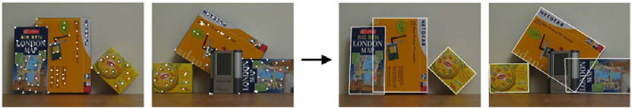
Fig. 7. (Left) 2D images with 83 points are detected via corner detection algorithm. Less than 50% of the point correspondences are accurate. (Right) The boundaries of the bodies and transformed boundaries with the estimated motion parameters. The estimation is almost perfect. Courtesy O. Tuzel.
