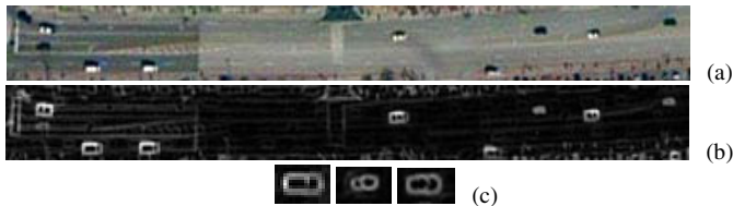
Fig. 6. (a) An original image. (b) The morphology preprocessing result. (c) Antibody examples.
