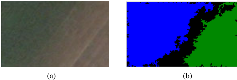
Fig. 2. (a) Original satellite image, (b) Segmented image using region growing
