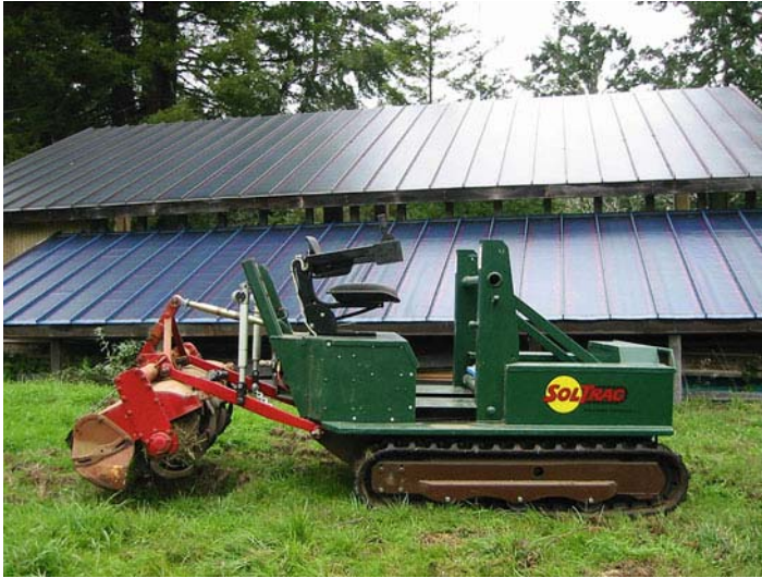
Fig. 7.1 Solar charged electric agricultural tractor designed and built by Stephen Heckerth, www.renewables.com
