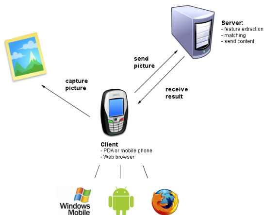
Fig. 1. High-level architecture of the prototype system
