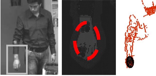
Fig. 3. Two-stage mean-shift procedure. Projected search region (left), 3D probability grid (middle), final result (right).
