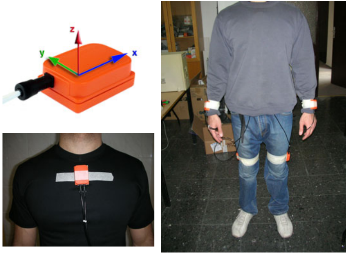
Fig. 1. Xsens sensor modules and their positioning on the body
