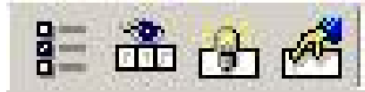
Fig. 1 Data Capturing Objects (Left to Right: Tick box Group, Handwriting Recognition Object, Manual Image Area, Automatic Image Area). Source: Formic Fusion Software
