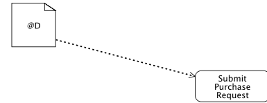
(i) (Q9): An association query between an activity and a variable data object
