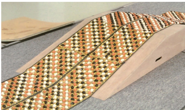
Fig. 1 Artificial uneven inclined walkway
