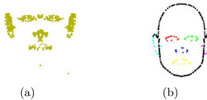
Fig. 5. An example of inner-contour extraction. (a) Points with high Gaussian curvatures. (b) The results of inner-contour extraction.
