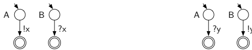
Fig. 5. Two pairs of peers which distributedly realize the choreography of Fig. 4(c)
