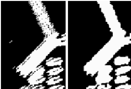
Fig. 5. Error regions before (left) and after (right) applying a median filter: one-pixel-regions are eliminated
