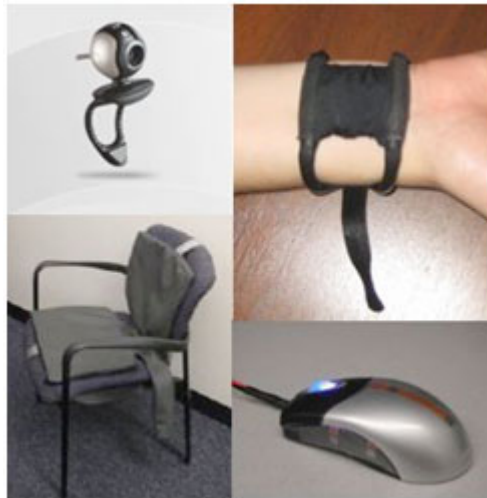
Fig. 10.1 Sensors used in the classroom (clockwise): mental state camera, skin conductance bracelet, pressure sensitive mouse, pressure sensitive chair.
