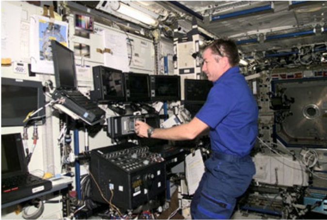
Fig. 8.3 Astronauts have to deal with three camera views and a complementary textual source of information for figuring out Canadarm's situation. NASA
