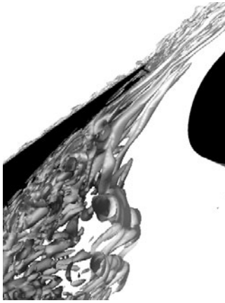
Fig. 7. Vortical structures in the reattachment area of the slat cover shear layer visualized by \lambda_2 contours.
