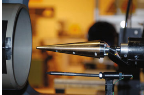
Fig. 1. Blunt nose cone model and Pitot probe in front of the Mach-6-nozzle
