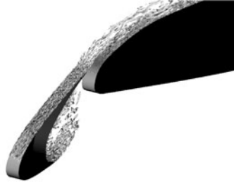
Fig. 5. Vortical structures in the slat area visualized by \lambda_2 contours with mapped on Mach number distribution.
