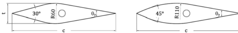
Fig. 2. Simplified drawing of the profile models: chord length c = 144.3 \text{ mm} , max. thickness t = 19\% of c , trailing edge apex angle \theta_2 = 20^\circ , the locations of max. thickness are 41% and 39% of c for the profiles with \theta_1 = 30^\circ and \theta_1 = 45^\circ , respectively.
