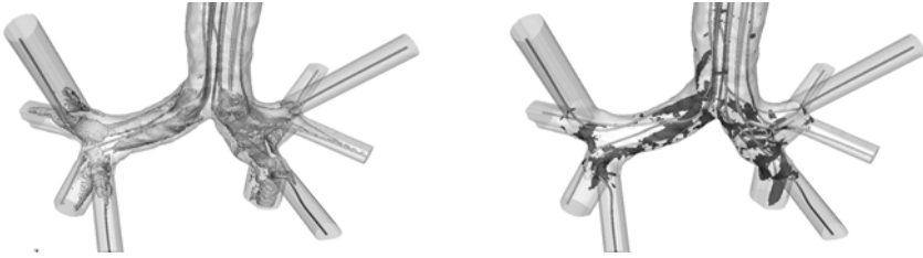
Fig. 1. Isosurfaces of normalised helicity (left) and vortical structures (right) of the constant flow in a 3rd generation lung model
