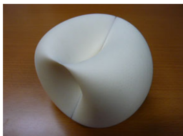
Fig. 12. Model 11: our original math surface constructed by selective laser sintering; height = 6cm
