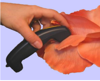
Fig. 2. Color identifier manufactured by BRYTECH [2]
