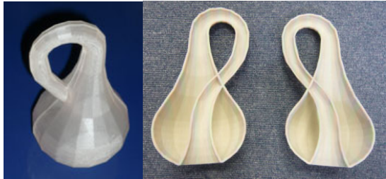
Fig. 4. Model 3: Klein bottle, Left: constructed by stereolithography, height = 10 cm, Right: constructed by 3D printing, height = 20 cm
