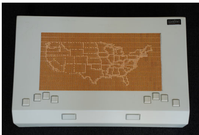
Fig. 1. A US state map (without Alaska) on BrailleDis 9000 (white dots are raised pins)
