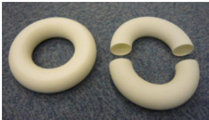
Fig. 5. Model 4: ring torus, constructed by selective laser sintering; d = 7.5 cm, r = 2.5 cm
