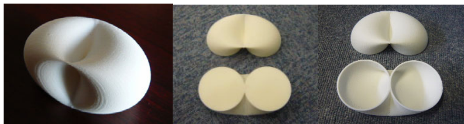
Fig. 11. Model 10: our original math surface constructed by selective laser sintering; Left: complete model, Middle: incorrect partitioned models, Right: corrected partitioned models, height = 6 cm
