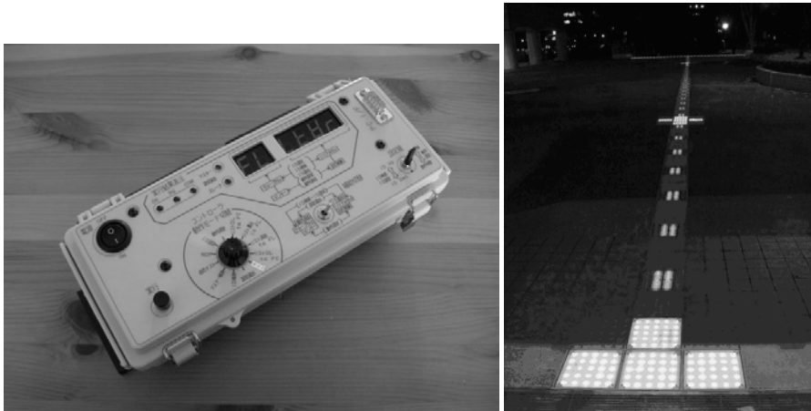
Fig. 2. Left photograph shows a remote control box. A computer writes a certain program to the box through a serial cable. The box stores the program and writes it to a Braille block via infrared. Right photograph shows an overview of light-emitting Braille blocks in the night. Levels of illumination is controlled in eight levels.
