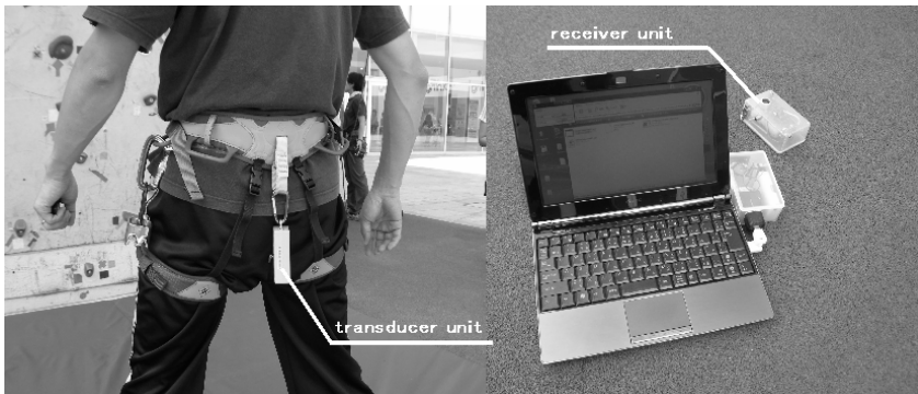
Fig. 2. A pair of ultrasonic device which measures distance between each unit. Left photo shows a transducer unit hung on a harness a climber wears. Right photo shows a PC and a receiver unit on the ground. The receiver unit and the PC connected using radio wave.
