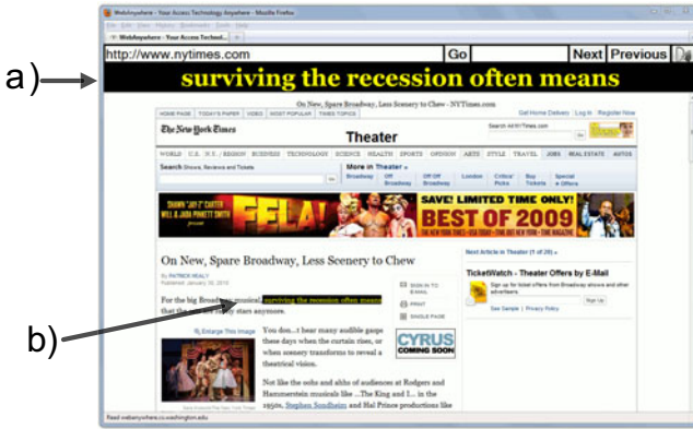
Fig. 2. The basic visualization. (a) The text currently being read is shown above the content in a high-contrast, magnified view to assist those reading along and those with low-vision. (b) The current content being read is highlighted so that users and developers can more easily read along with WebAnywhere.
