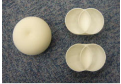
Fig. 8. Model 7: spindle torus, constructed by selective laser sintering; d = 1.25 cm, r = 2.5 cm
