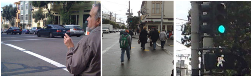
Fig. 1. Overview of proposed Crosswatch system. Left to right: (a) Blind pedestrian holding mobile phone. (b) Image of crosswalk taken from across the street. (c) Zoomed-up area of (b) shows Walk light visible at the end of the crosswalk. Proposed system is programmed to generate audio alert when Walk light is detected.
