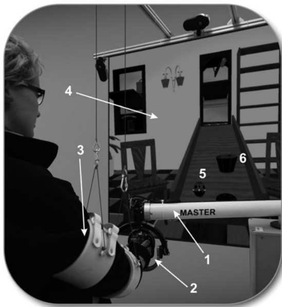
Fig. 1. A subject performing the virtual rehabilitation task. The subject performs the task using the robot (1) and grasping device (2) while his/her arm is supported by cuffs (3). The screen (4) shows a sloped table, a ball (5) and a basket (6).
