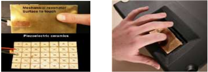
Fig. 1. The friction controlled tactile plate for rendering spatial texture
