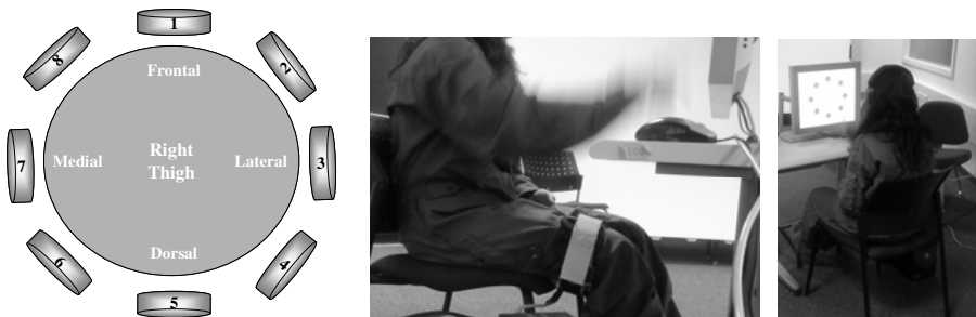
Fig. 1. Left: Midsagittal cross section of thigh (gray ellipse) and relative location of tactors (gray disks). Center: Positioning of the participant and apparatus. Elastic tactile belt mounted on right thigh. Right: Virtual buttons (circles) displayed on the touch screen.
