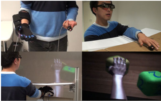
Fig. 1. VE for study the body ownership illusion of a virtual hand/arm with vibrotactile stimulations
