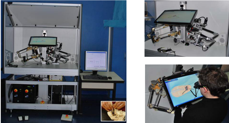
Fig. 2. The multimodal VR training platform is an autonomous mobile cabinet including two 6 DOFs haptic devices equipped with an active tactile drill prop and a passive vacuum cleaner prop, a tangible support figuring the chin of the patient, a 3D screen with stereoscopic glasses, a head mocap system, and 2 loudspeakers. The lower rack integrates the haptic devices controllers, the main PC running the application, the active prop amplifier and the audio sound card. An additional screen is used to display performances feedback.
