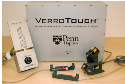
Fig. 2. The components of the VerroTouch system when not installed on a da Vinci surgical system. From left to right, one can see the gain control module, two vibration sensor clips, and two vibration actuator clips. The main receiver box is shown at the back.
