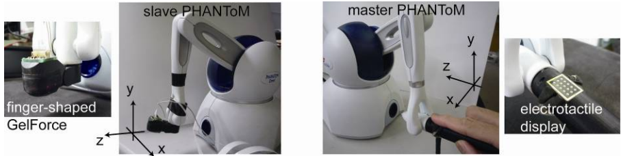
Fig. 3. Experimental setup: one-fingered transmission system for spatially distributed tactile information employing PHANTom master-slave system
