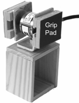
Fig. 1. The apparatus used in the experiments consisted of a force transducer attached to the top of a box in which different weights were loaded
