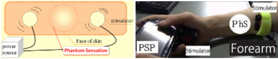
Fig. 1. PhS is induced by tactile stimuli in two locations. The location in which PhS is experienced is determined by the ratio between the strength of the two stimuli. The image on the right shows an example of one potential application of PhS. This system stimulates the palm and forearm, in conjunction with a handheld videogame. PhS can be elicited at any location of the forearm with a very simple setup, and could be used to produce tactile sensations as part of a videogame.
