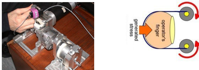
Fig. 1. Shot of the prototype, including the joystick and the tactile device (left). Scheme of the tactile device: two motors allow to generate a stress normal to fingertip (right).
