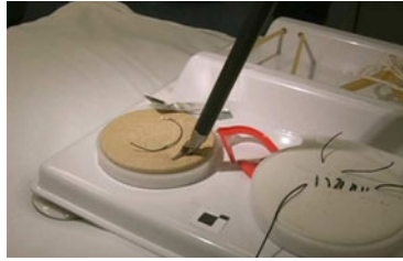
Fig. 4. The manipulation environment chosen for testing. The operator used a large da Vinci needle driver to interact with the practice suture pads, suture needles, small objects, rubber tubes, soft strings, and the hard plastic structure of the task board.
