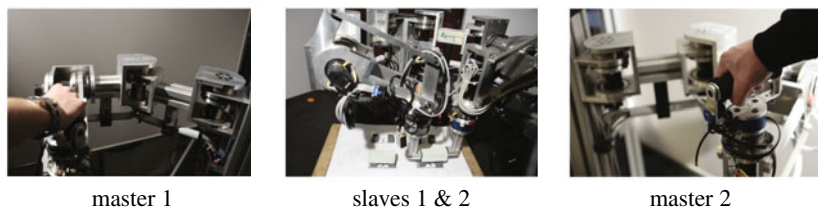
Fig. 2. Experimental Setup: One partner controlled the left teleoperator arm (slave 1) by using the haptic interface depicted on the left (master 1) while the other partner controlled the right teleoperator arm (slave 2) by using master 2
