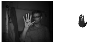
Fig. 6. Out of pose space gestures are incorrectly estimated. Left: ToF amplitude image with superimposed skeleton estimation. Right: Corresponding range image.
