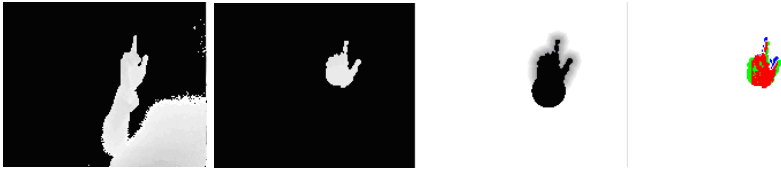
Fig. 3. The measurement of one particle hypothesis. Left to right: The preprocessed input X , The particle Z_k range image, Z_k 's neighbourhood region in grey and classified image with correct, false and missed pixels indicated with red, green and blue.
