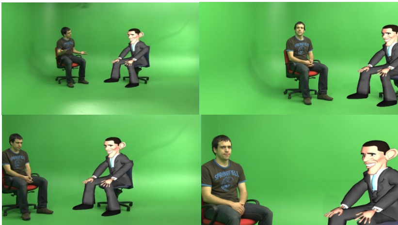
Fig. 4. Playing with the real camera parameters: changes in translation and zoom (chroma system is not necessary; it is just for having a clean background. Virtual character’s chair is real, non virtual).
