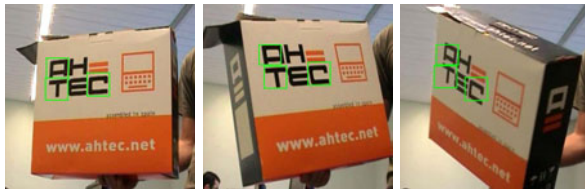
Fig. 5. Sequence showing frames 1, 89 and 123 where a rotation out of the image plane is present
