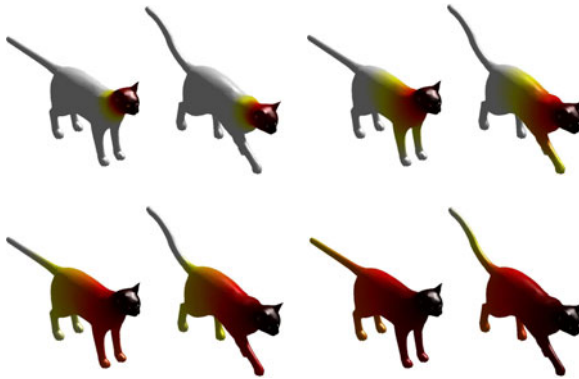
Fig. 4. The average diffusion distance for the tip of the nose to all other points is shown for different diffusion times
