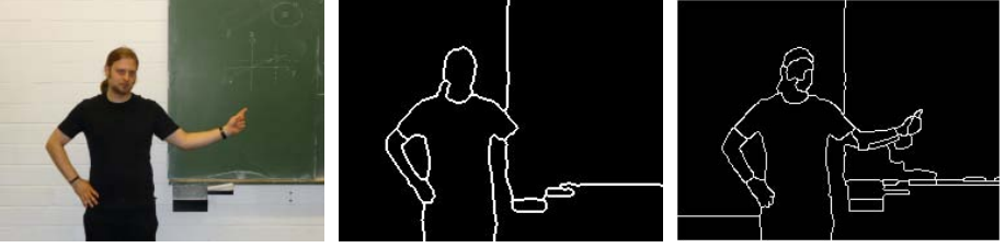
Fig. 2. Results of JSEG (center) and EDISON (right) edge segmenters on the image on the left; parameters are chosen according to [18] and [19], respectively
