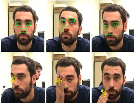
Fig. 2. Upper row: On the left, initialization of both trackers. The central and right image shows frames 78 and 234 for the case of the joint state space (12 dimensions). Lower row: Each part is tracked individually. The green stars show the estimated position. The left image shows how the right eye tracking is totally lost (draught by the hand) after the partial occlusion.
