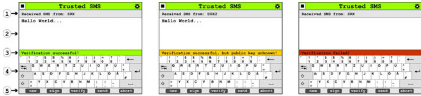
Fig. 5. Screenshot of the TrustedSMS application indicating the different trust states of an SMS
