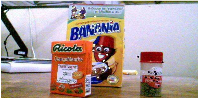
Fig. 3. Keypoints corresponding to different recognized objects: box of chocolate milk mix (full white circles), box of sweet (empty circles), pepper pot (full black circles).
