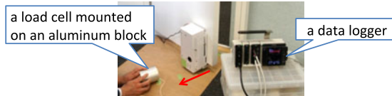
Fig. 9. Snapshot of collision detection experiment
