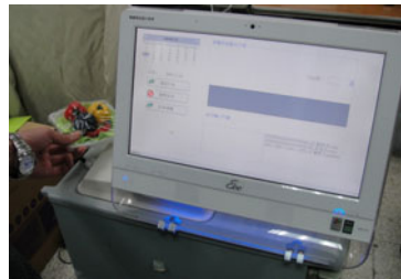
Fig. 7. Smart refrigerator attached with an RFID reader and a touch screen
