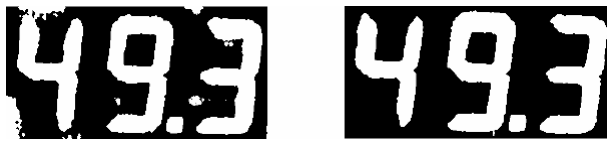
Fig. 9. Images binarized with interpolated thresholds. Left: 8x8 sub-images. Right: 4x3 sub-images.
