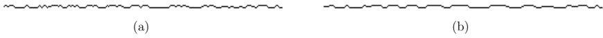
Fig. 4. Smoothing Pixel-Paths: (a) the original pixel-path resulting out of a texture stripe (b) the smoothed pixel-path where t is set to 4. That is, all peaks in the y -direction lying within a range smaller than 4 are discarded.
