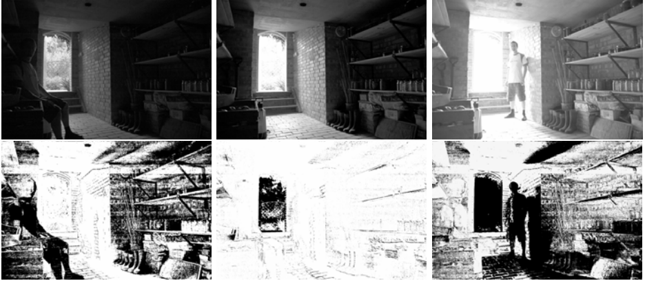
Fig. 4. Example LDR images sequence (top row: \frac{1}{640}s , \frac{1}{160}s , \frac{1}{40}s ) and their normalized ghost maps (bottom row)
