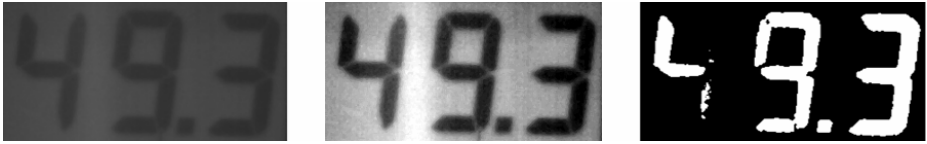
Fig. 8. Left : Image with illumination gradient (not very evident, more visible in an equalized image: middle ). Right : binarization with a single threshold.
