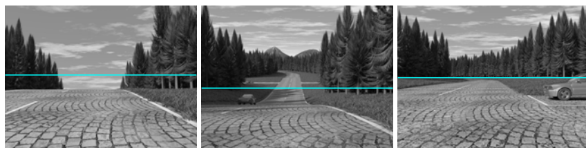
Fig. 6. Horizon lines computed by the proposed approach on a synthetic video sequence illustrating different situations: uphill, downhill and flat roads
