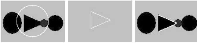
Fig. 1. Segmentation on synthetic image: (a) Original image with initial contour; (b) Prior shape; (c) final result
