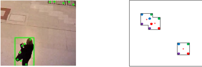
Fig. 1. Left: Example for “Good Features To Track” (Picture from PETS 2006). Right: marker scheme for features: (cross: feature point, blue: 2, green: -2, violet: 1, red: -1) and area for which integral images have to be built.
