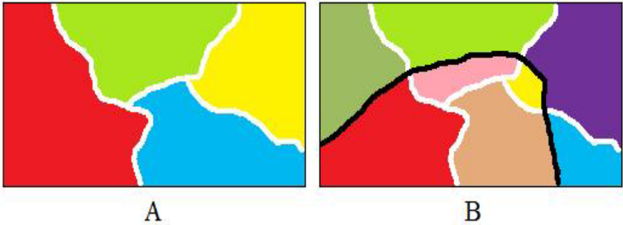
Fig. 2. A) Watershed over-segmentation: the white lines are the watershed lines separating regions, and the total number of regions is 4. B) Combining edge line: black line is a detected edge line, and the total number regions after combining the edge line is 8.
