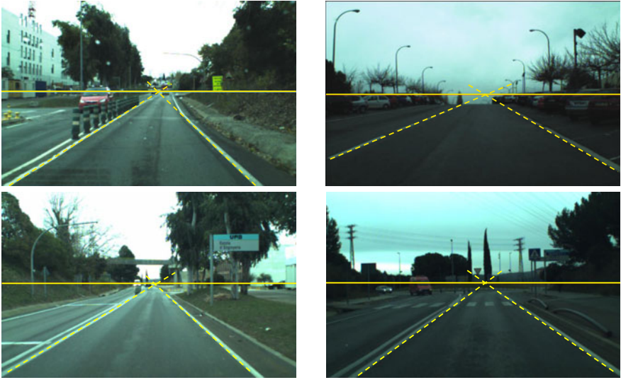
Fig. 9. Real video frames with the horizon lines estimated by the proposed approach (note that they correspond with the intersections of the projected lane markings)
