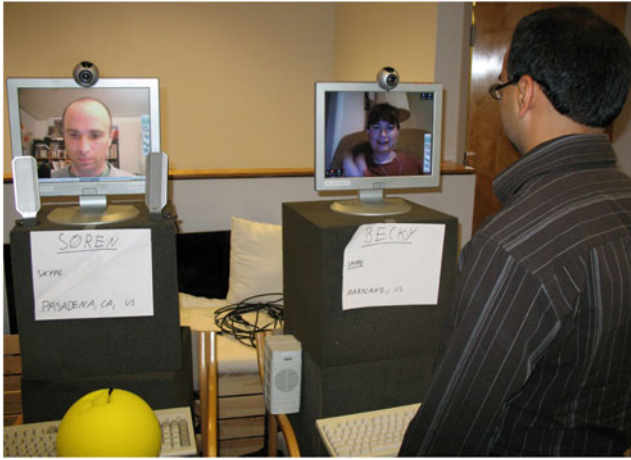
Fig. 3 Early physical avatars. This image shows two distant participants speaking with a local moderator by video chat. Their screen images are positioned atop kiosks at eye-level, and each has a personal camera, microphone and speaker for close-up conversation. Their names, location in the world, and instant messaging identity are shown so local participants can join them in the back-channel chat. A foam microphone ball, passed around by local speakers during Q&A dialog, is visible at the bottom left
