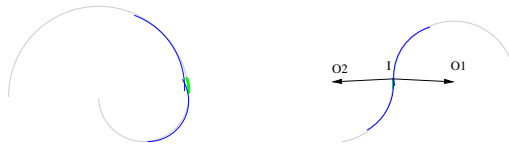
Fig. 5. Intersection of arcs with opposed curvature signs or with significantly different radii
