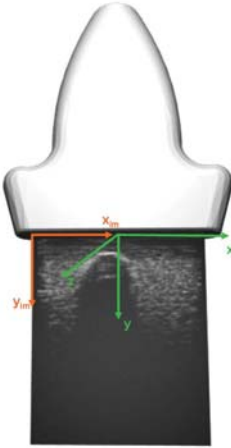
Fig. 3. Definition of local 2D and global 3D ultrasound image coordinate system
