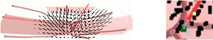
Fig. 6. Left: Needle insertion simulation along a path P . Right: zoom on the target.
