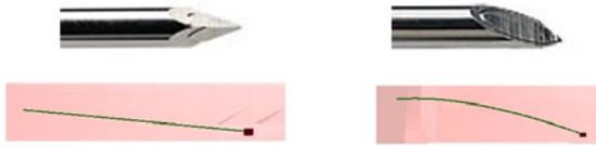
Fig. 3. Trajectories generated by non-steerable needles (orientation fixed). Left: a symmetric rigid needle follows a straight line. Right: a bevel-tip flexible needle follows an arc of circle.
