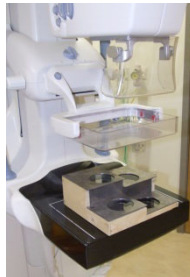
Fig. 1. The phantom used for calibration of the family of detector transfer functions
