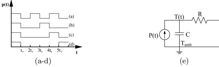
Fig. 1. Power profiles for (a) x = 2 , (b) x = 3 , (c) x = 4 , and (d) x = 5 . (e) shows the RC thermal model.
