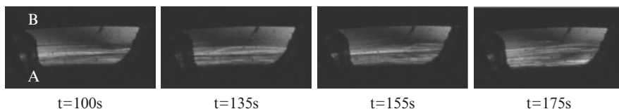
Fig. 24 Illustration of fluctuating behavior of the banding structure on long time scale. The sample, made of C_{16}TAB (0.3 M) and NaNO_3 (1.79 M) ( c = 11 wt. %) is sheared at \dot{\gamma} = 8 \text{ s}^{-1} in the annular gap of a Couette cell placed between crossed polarizers and illuminated by a source of white light. The temperature is fixed at 30^\circ\text{C} . The observation is realized in the (\mathbf{v}, \mathbf{V}_v) -plane. The inner rotating cylinder and the outer fixed wall of the Couette cell are indicated by the letters a and b , respectively. Reprinted from Lerouge et al. [144]
