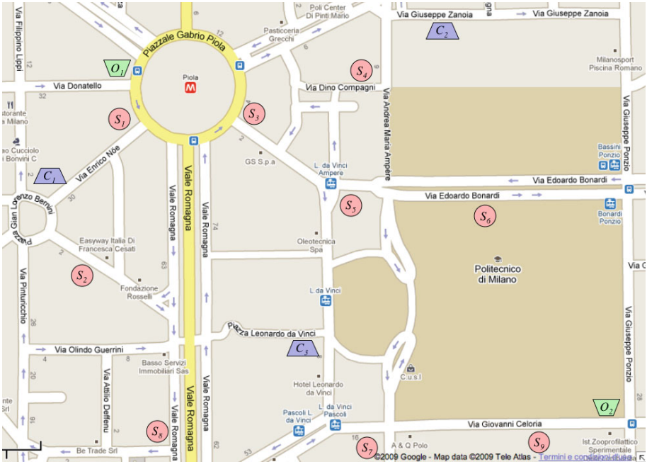
Fig. 1. Micro example on the Politecnico of Milano campus, with two candidate sites for the central offices O_i (downward trapezia), three candidate sites for the cabinets C_j (upward trapezia), and nine basements S_l (circles)
