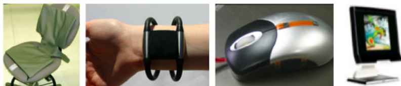
Fig. 2. Affective sensors (from left to right): posture chair, skin conductance (SC) bracelet, pressure mouse, Tobii eye tracker
