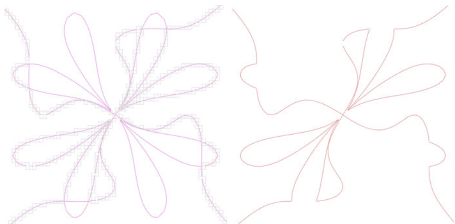
Fig. 7. Left: defining curves and cell graph. Right: boundary contours of the underlying set.
