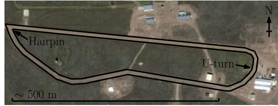
Fig. 6 The 1.3-kilometre test track used for field trials. The track is a gravel road and is approximately 7 metres wide. The most difficult portions of the track are the U-turn and the hairpin turn.
