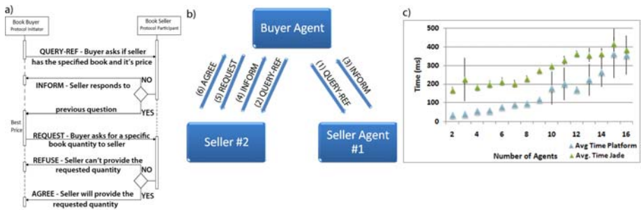
Fig. 4. Book buyer and book seller agents' protocol, a). An example of message exchange in this test scenario with seller #2 providing the book's best price, b). Test's results for Jade and the described platform, c).
