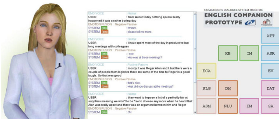
Fig. 1. Overview of the system interface featuring the ECA and including a real-time transcript of the whole dialogue, including output from the emotional speech recogniser. In this example, the dialogue is clearly led by the user (user utterances are displayed in a black font).
