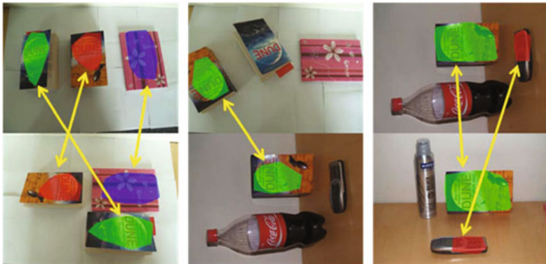
Fig. 6. Pairs of affine-related regions detected in exemplary images. Note that some regions are only approximately planar.
