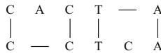
Fig. 1. This example shows the similarity matrix H computed for a query sequence A = AGCCTCA and a target sequence B = CACTATGC using Smith-Waterman algorithm. And tracing back from the maximum value of the similarity matrix ( H(7, 5) = 6 ), we can get the pair of most similar subsequences: CACTA and CCTCA .
