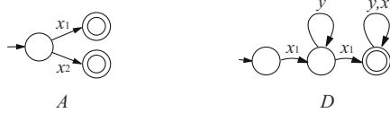
Fig. 2. A nondeterministic VFA whose pattern automaton is deterministic, and a DVFA that accepts all words in which the first letter is repeated at least twice
