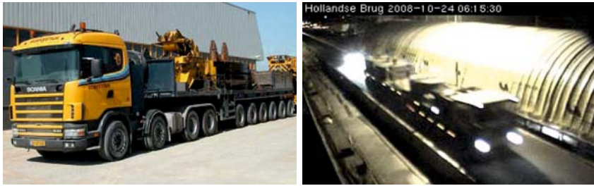
Fig. 3. The 10 axle test truck that was driven across the bridge in the early morning
