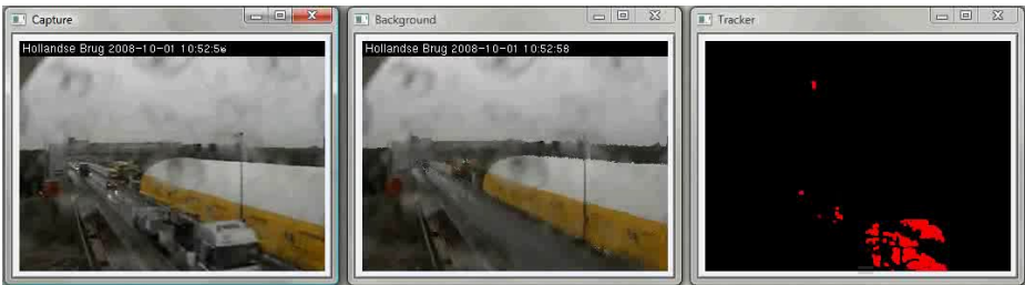
Fig. 6. Estimating large blobs of moving objects: (left) the input image, (middle) the expected background over the recent past, (right) the estimated location of moving objects
