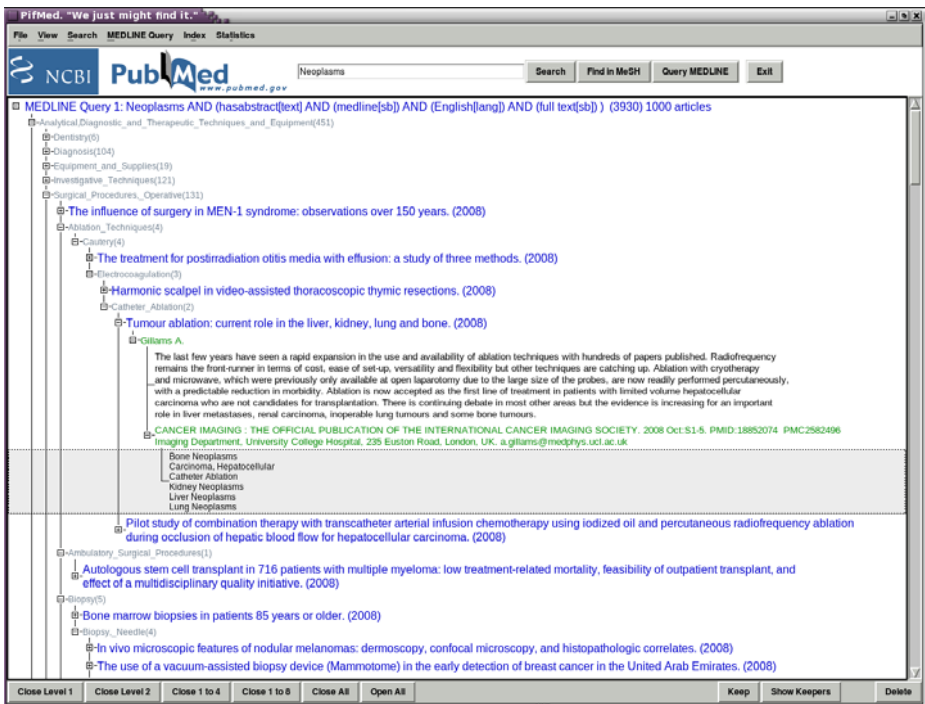
Fig. 2. A screenshot of the MeSHLINE user interface. The root of the tree is the MEDLINE query in full. In brackets following the root is the total number of title nodes in the tree, following the total number of title node is the total number of articles. These are not equal because most articles have more than one MeSH term attributed to them. The grey text are MeSH terms, organized into a hierarchy. The blue nodes within the tree are title nodes. Inside a title node is a green author node. Inside the author node is an abstract in black, followed by the bibliographical information. The child of the green bibliographical node is a list of the MeSH keywords attributed to a given article.
